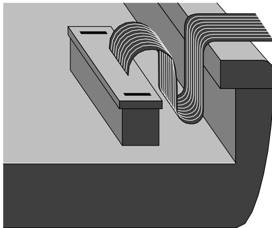
Figure 25 - Proper Keyboard Flex Cable Position
